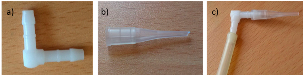
Figure 8. (a) Elbow connector, (b) cone-shaped connector, and (c) large section tube with both connectors.
