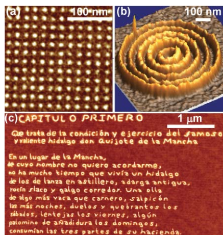
Fig. 4 Examples of local oxidation nanopatterns. (a) Periodic array of 10 nm silicon oxide dots. The lattice spacing is 40 nm. (b) Alternating insulating (bright) and semiconducting rings. (c) First paragraph of ‘Don Quixote’.
