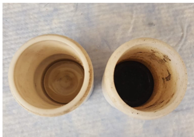
Figure 1 Solutions of GREEN-TeNWs after the reaction. The colorless solution without starch (left) and dark solution containing starch (right).
