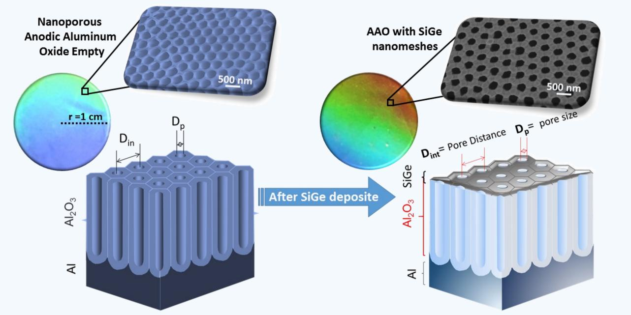
The sputtered  $Si_{0.8}Ge_{0.2}$  films replicated the porous alumina matrices (AAO) highly oriented structure, resulting in the nano-meshed films with different pore sizes. This fabrication process allows growing large areas of  $Si_{0.8}Ge_{0.2}$  nano-meshed films in a simple and reliable way, and can be easily industrially scalable.
