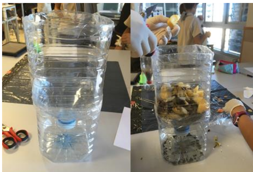
Figure 1. Construction of a small-scale composting reactor used in this experiment.
