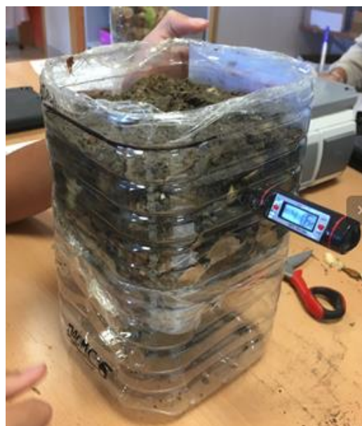
Figure 3. Measuring temperature in a small-scale composting reactor.
