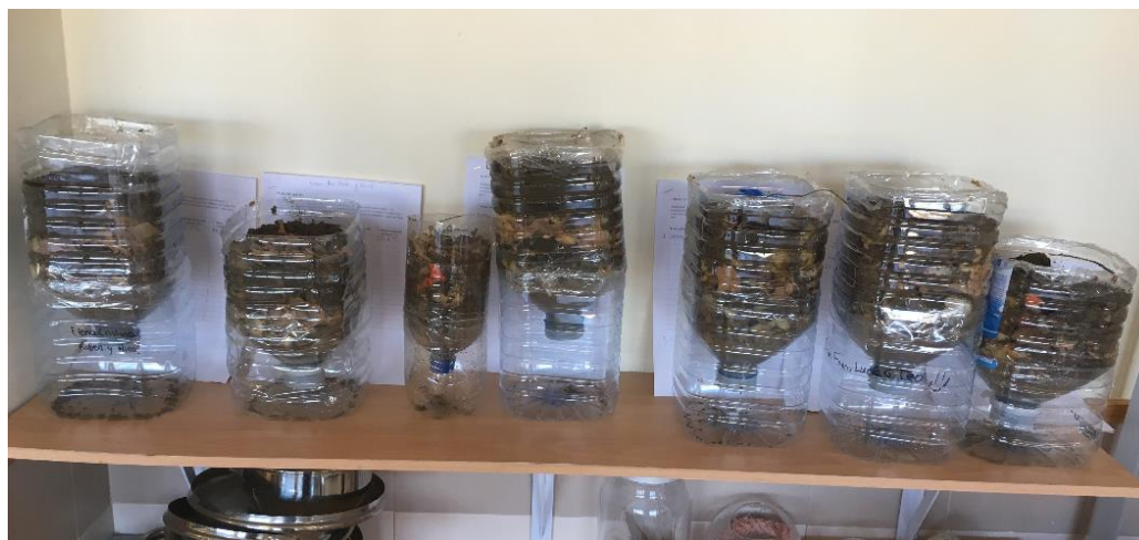
Figure 2. Small-scale composting reactors used at the beginning of the process.
