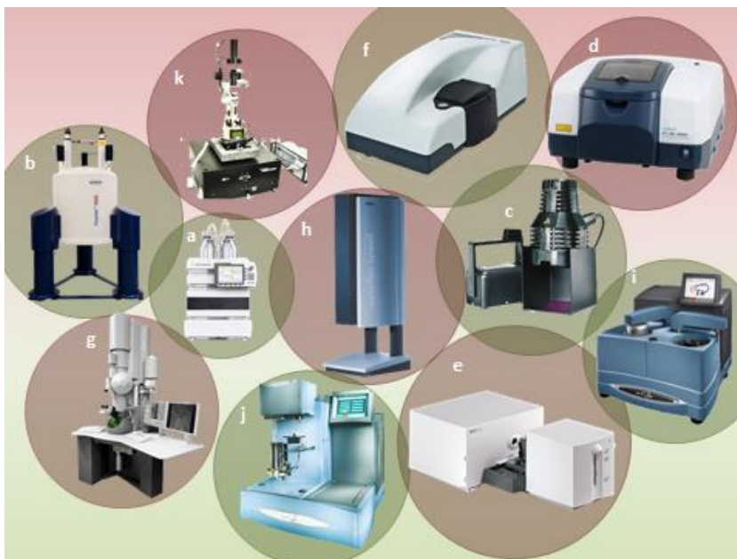
Figure 5.1.1: Pictures of different instruments. Size exclusion chromatography (a), Nuclear magnetic resonance spectroscopy (b), UV-Light source (c), Fourier transform infrared spectroscopy (d), Ultraviolet/Visible spectroscopy (e), Dynamic light scattering (f), Transmission electron microscopy (g), Matrix-assisted laser desorption/ionization (h), Differential scanning calorimetry (i), Thermogravimetric analysis (j).
