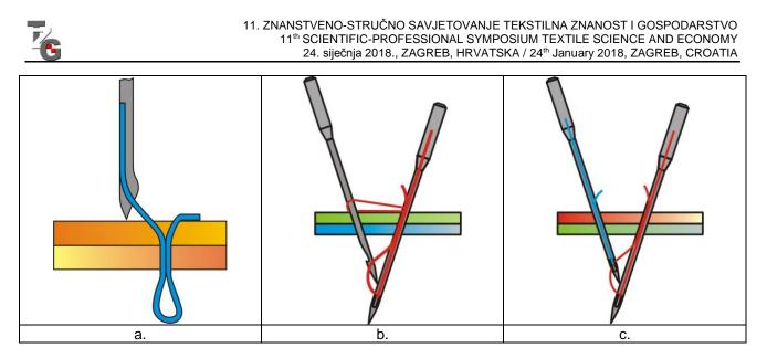
Figure 2: One side stitching, a. tufting, b. two needle - one thread, c. two needle - two thread
