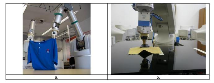
Figure 1: Handling with robot, a. mechanical grasping of cloth, b. vacuum grasping of textile material
