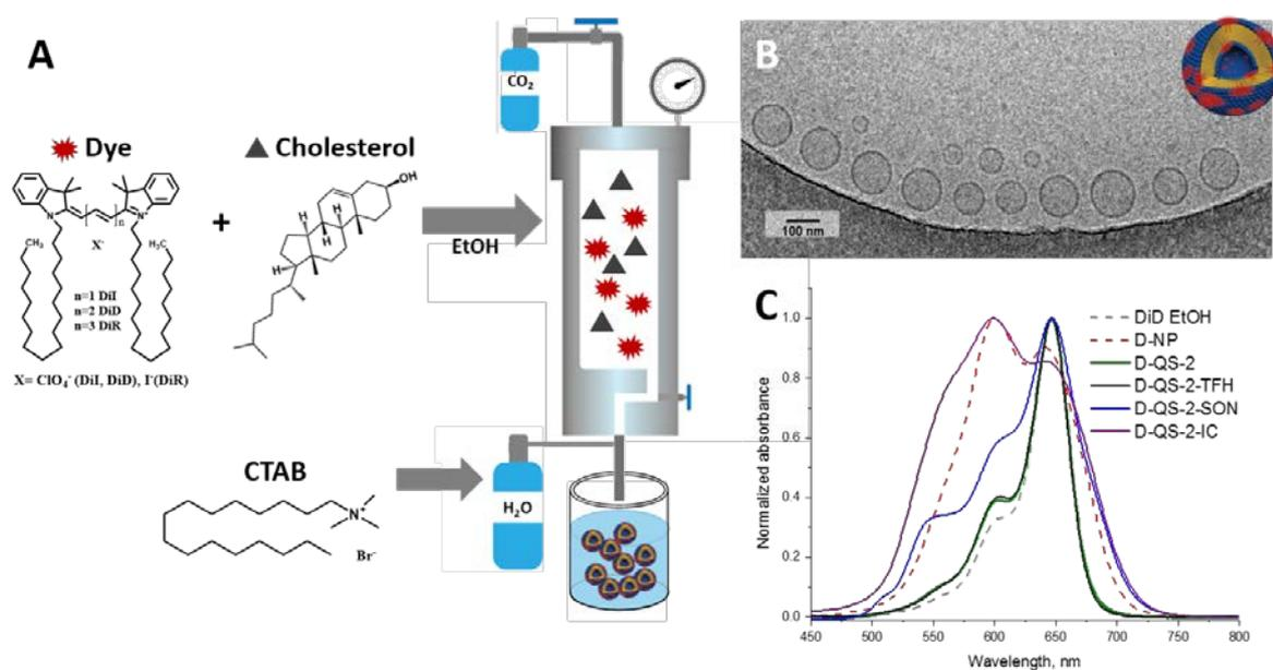
**Figure 1.** A) Schematic representation of DELOS-SUSP method for the preparation of Quatsomes loaded with dyes (DiI, DiD and DiR). B) CryoTEM image of D-QS-2 and C) absorption spectra of DiD in EtOH, DiD-based NPs and D-QS prepared by different methods (see Text).
