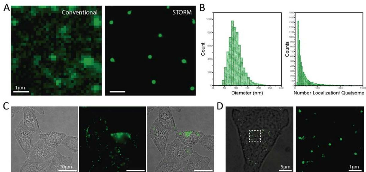
**Figure 4.** A) Images of DiI-loaded Quatsomes (I-QS-1) obtained by conventional wide-field microscopy and STORM ( $\lambda_{exc} = 561$  nm). B) Distribution of size and number of localizations per Quatsomes extrapolated from STORM images. C) Snapshot of the video (see SI) acquired by fluorescence microscopy of the internalization of QSs in HeLa cells. D) STORM images of QSs internalized in HeLa cells.
