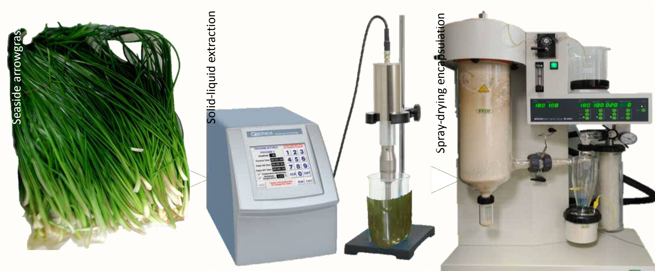
Figure 3: from left to right, Seaside arrowgrass, Sonication-favoured extraction and spray drying equipment used for microencapsulation
