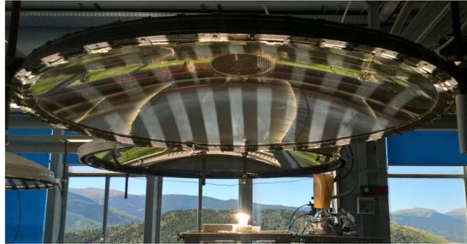
Fig. 1. Parabolic solar concentrator.
