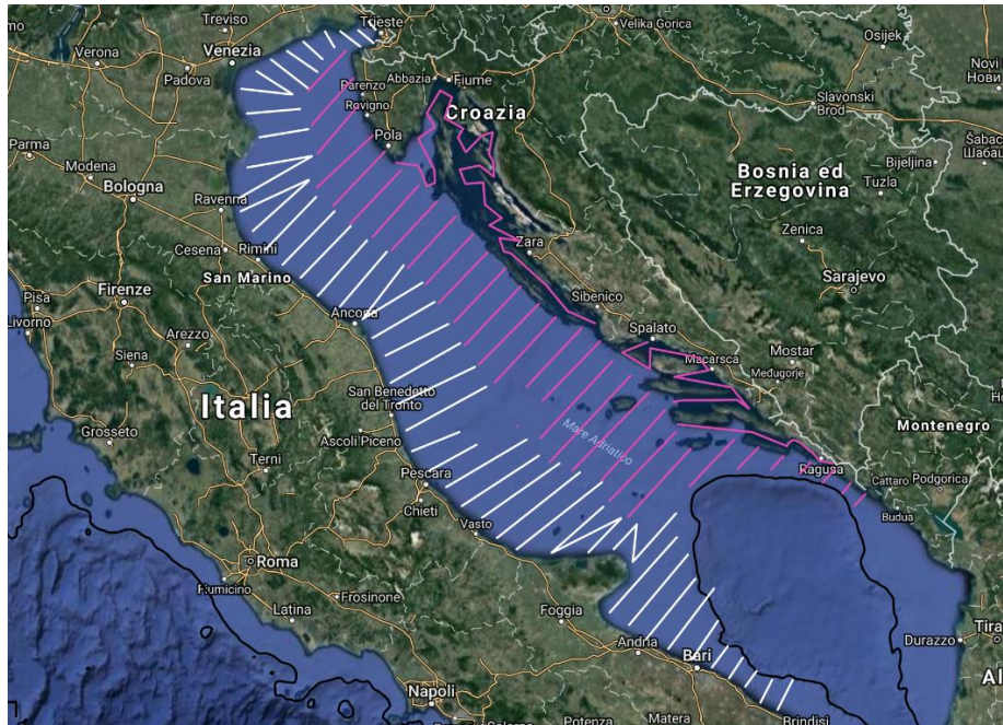
Figure 6.6.4.1. Acoustic transects for the western echo survey (white tracks) and the eastern echo survey (pink tracks) for the GSA 17 and GSA 18.
