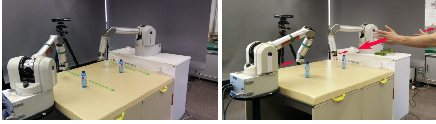
Fig. 2: A user guiding dual-arm robot using hands motions tracked by Kinect camera. Left: the initial trajectory is shown in green. Right: red arrows represent the motions of both user hands and robot end-effectors in the teleoperation mode.
