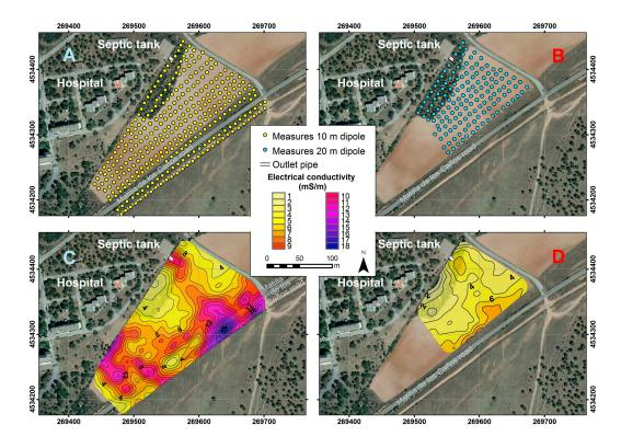
**Figure 4.** Meshing of sampling points for the separation between the coils of 10 m (**A**) and 20 m (**B**). Electrical conductivity maps obtained with a horizontal dipole (vertical coils) with a spacing of 10 m (**C**) and 20 m (**D**).
