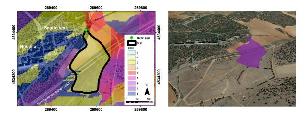
**Figure 6.** Delimitation of effluent discharge using GIS techniques based on a cost–distance algorithm (**left**) and 3D (three dimensional) modeling with an ArcScene script (**right**).
