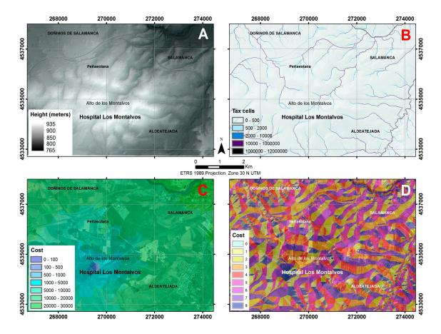
**Figure 3.** Methodological sequence with GIS (Geographic Information System) technique: digital elevation model (**A**), drainage network (**B**), accumulated costs (**C**) and possible routes map (**D**).
