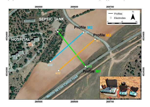
**Figure 5.** A. Location of acquisition of three profiles M1, M2 and M3. The inset shows the PASI 16SG24-N resistivimeter, the energizer and the two link boxes.
