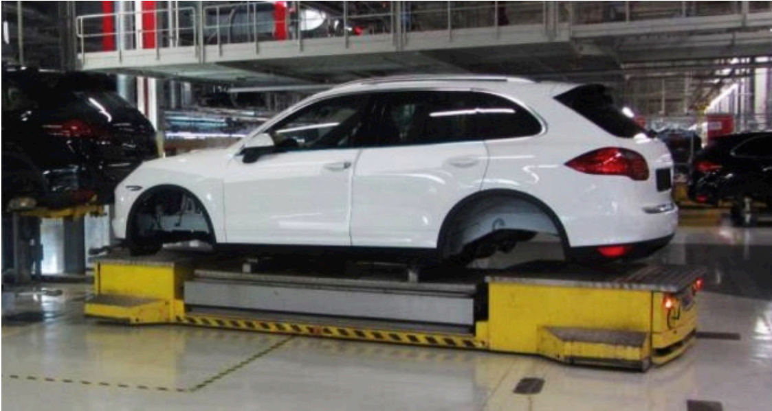
Figure A.12 MAX AGV Porsche Final Assembly Line AGV [12]
