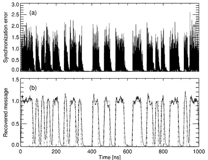
Fig. 8. ON/OFF phase shift keying encryption scheme. (a) Synchronization error defined in (7). (b) Recovered digital message at 64 Mb/s after a filtering process. Parameters:  $\kappa_t = \kappa_r = 20 \text{ ns}^{-1}$ ,  $\kappa_c = 30 \text{ ns}^{-1}$  and  $p_t = p_r = 1.5$ .
