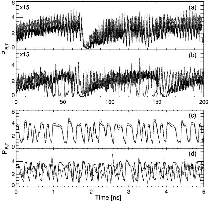
Fig. 5. Temporal evolution of the optical power  $P_{T,R} = |A_{T,R}|^2$  in the: (a), (b) LFF regime  $p_t = p_r = 1.0$  and (c), (d) CC regime  $p_t = p_r = 1.5$ . Solid lines: transmitter. Grey lines: receiver. Parameters: (a), (c)  $\kappa_t = \kappa_c = \kappa_r = 20 \text{ ns}^{-1}$ ,  $\alpha = 4$ ,  $\Delta\Phi = 0$  and (b), (d)  $\Delta\Phi = \pi$ .
