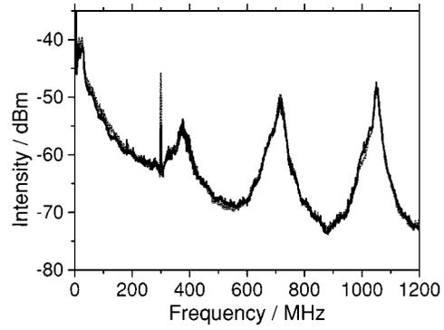
Fig. 4. Experimental RF spectra of the synchronized ( $\Delta\Phi = 0$ ) transmitter signal (grey line), and receiver signal (black line) under LFF operation ( $I_{t,r} = 1.01 I_{\text{th,soI}}$ ) showing the response of the subsystems on small sinusoidal modulation of the transmitter. The frequency of the modulation is 300 MHz, and the amplitude is  $0.01 I_{\text{th,soI}}$ .
