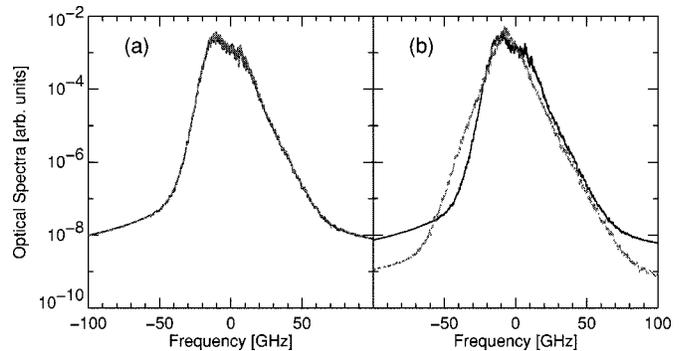
Fig. 7. Calculated optical spectra of the transmitter (black lines) and receiver (grey lines) when (a)  $\Delta\Phi = 0$  and (b)  $\Delta\Phi = \pi$ . Parameters:  $\kappa_t = \kappa_r = \kappa_c = 20 \text{ ns}^{-1}$ , and  $p_t = p_r = 1.5$ .
