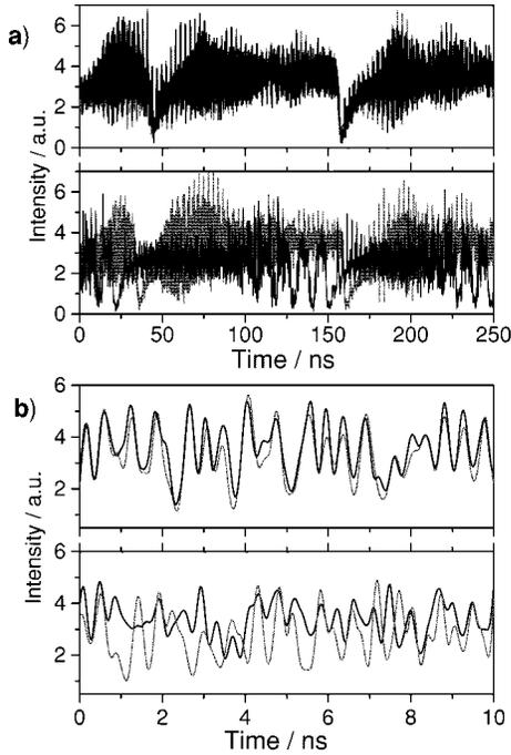
Fig. 2. Synchronization behavior of transmitter intensity (grey line), and receiver intensity (black line) in dependence on the relative optical feedback phase  $\Delta\Phi$ . (a) LFF operation with  $I_{t,r} = 1.01 I_{th, sol}$ . (b) CC operation with  $I_{t,r} = 1.15 I_{th, sol}$ . The upper panels in each subplot correspond to adjusted phase  $\Delta\Phi = 0$ , the lower panels correspond to  $\Delta\Phi = 0.7\pi$ .
