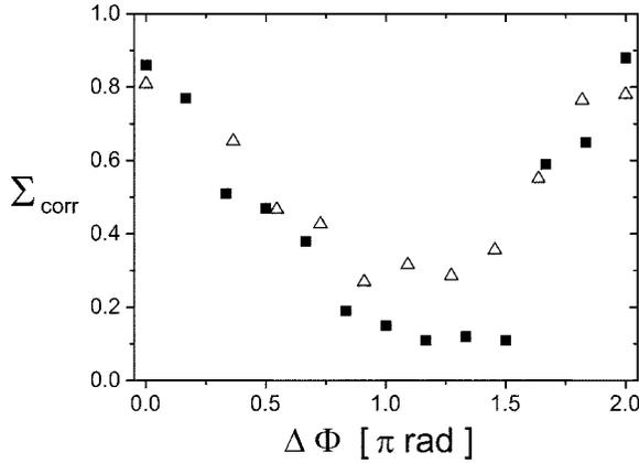
Fig. 3. Experimental cross-correlation coefficients of the intensity time series of transmitter and receiver versus the relative optical feedback phase  $\Delta\Phi$  under LFF operation ( $I_{t,r} = 1.01 I_{\text{th,soI}}$ , solid squares), and CC operation ( $I_{t,r} = 1.15 I_{\text{th,soI}}$ , open triangles), respectively.
