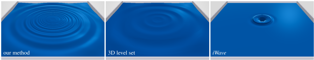
Figure 2: A 10-meter-wide and 1-meter-deep domain is perturbed, and we compare the resulting waves with our method (left, on a 256 \times 256 2D grid), a 3D level set simulation [Thuerey and Pfaff 2016] (middle, on a 256 \times 256 \times 128 3D grid), and the iWave method [Tessendorf 2004a] (right, also on a 256 \times 256 2D grid). All images show the simulation after 6 seconds. The difference in wavefront propagation velocity between our method and the level set solution is only 4.1%. However, our method runs at 30 fps and the level set solution runs at 20 seconds/frame (although it could be further optimized). Moreover, due to numerical dissipation, the level set solution misses the high-frequency waves, which are in turn captured with our method. iWave considerably underestimates the propagation velocity.
