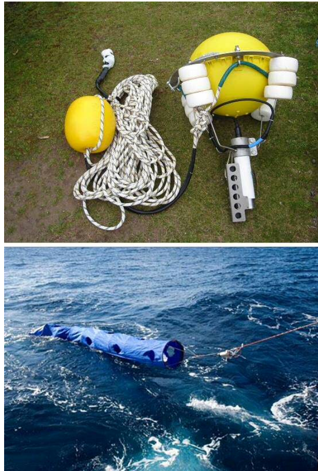
Fig. 6. – Top: drifter configuration with an external probe and tension-connecting elements for sampling at a nominal depth of 0.5 m. The 15-m rope leads to the drogue. Bottom: configuration for subsurface sampling where sensors are located at the mouth of the holey-sock drogue and the rope is replaced by a tension-holding energy and data transmission cable. The picture corresponds to the deployment of a 100-m depth drifter.
