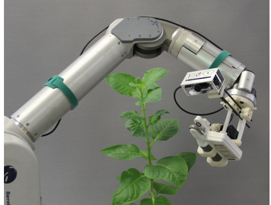
Fig. 1: Example of an eye-in-hand configuration, with a ToF camera attached to the manipulator end-effector, in this case a Chlorophyll meter.
