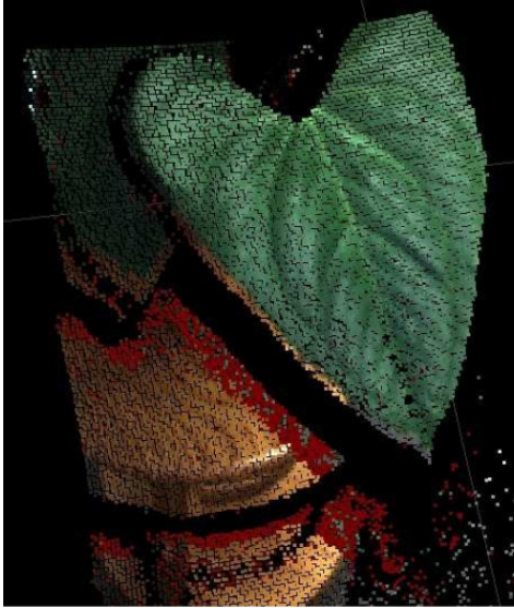
Fig. 6: Calibration errors produce bad colored points at the edge of the leaf. Additionally, observe the wrong color assignment in some background points, marked automatically in red, corresponding to the shadow of the leaf. This problem arises as the optical axes of the depth camera and the color camera are not the same and some depth points have no correspondence in the color image. Other sensor combinations, like Kinect, suffer the same problem.
