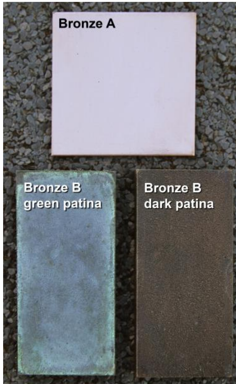
Fig. 2. Bronze coupons used for the electrochemical tests: clean bronze A (top), and artificially patinated bronze B, with a dark potassium sulfide patina (bottom right) and a green ammonium chloride patina (bottom left).
