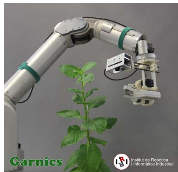
Setups for robot perception and manipulation of deformable objects at IRI (CSIC-UPC): a) perceiving and handling clothes [9,10,12], b) measuring the chlorophyll of plant leaves for phenotyping [7,8].
