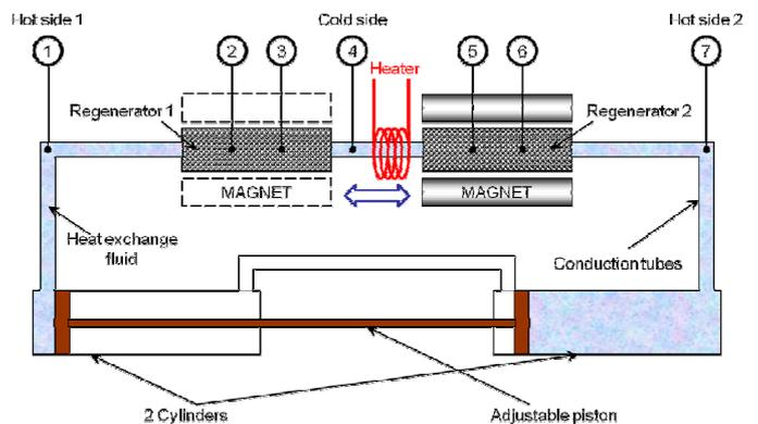
Fig. 1. Scheme of the magnetic refrigeration demonstrator. Temperature measurement points are indicated by numbers.
