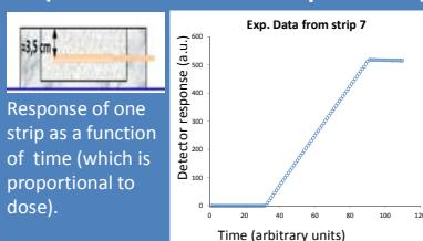
Irradiation with a 10cm x 20cm field and a source to surface distance (SSD)=100 cm. Detector is positioned as shown in the figure above.
