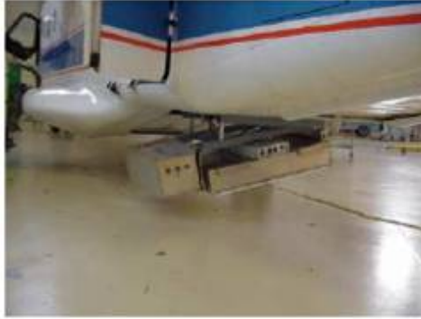
Figure 2.11: STARRS instrument installed on a DLR plane.
