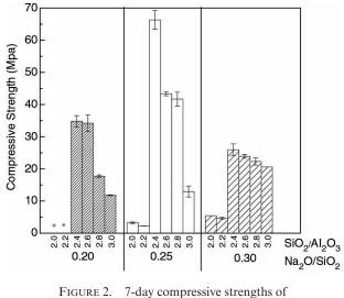
FIGURE 2. 7-day compressive strengths of alkali-activated SFCC specimens.
