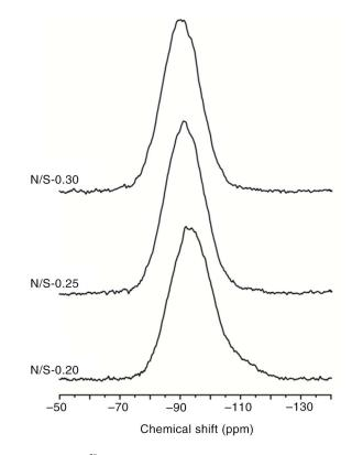
FIGURE 8. <sup>29</sup>Si MAS NMR spectra of SFCC geopolymers formulated with a SiO<sub>2</sub>/Al<sub>2</sub>O<sub>3</sub> ratio of 2.4, as function of the Na<sub>2</sub>O/SiO<sub>2</sub> (N/S) ratio.
