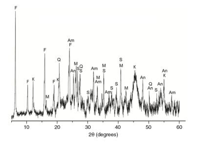
FIGURE 1. Diffractogram of the unreacted spent FCC catalyst. An: andalusite, Am: analcime, F: faujasite, K: kyanite, M: mullite, Q: quartz, S: sillimanite.
