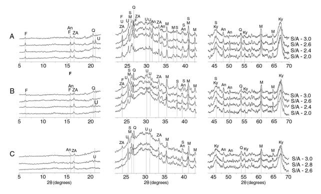
FIGURE 3. Diffractograms of activated SFCC pastes formulated with a Na<sub>2</sub>O/SiO<sub>2</sub> ratio of (A) 0.20, (B) 0.25 and (C) 0.30. An: analcime, F: faujasite, U: ussingite, ZA: zeolite Na-A, Q: quartz, M: mullite, S: sillimanite and Ky: kyanite.
