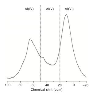
FIGURE 5. <sup>27</sup>Al MAS NMR spectrum of the unreacted SFCC.
