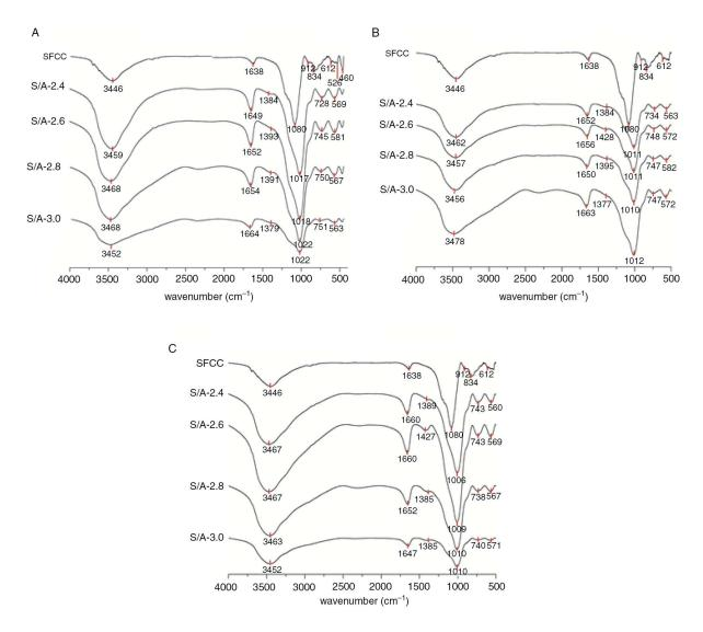
$\begin{array}{lll} \mbox{FIGURE 4.} & \mbox{FTIR spectra of SFCC precursor, and activated pastes formulated with $SiO_2/Al_2O_3$} \\ & (S/A) \mbox{ ratios as marked, at $Na_2O/SiO_2$ ratios of (A) 0.20, (B) 0.25, (C) 0.30.} \end{array}$
