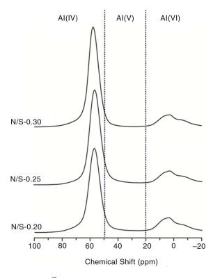
FIGURE 7. <sup>27</sup>Al MAS NMR spectra of SFCC geopolymers formulated with a SiO<sub>2</sub>/Al<sub>2</sub>O<sub>3</sub> ratio of 2.4, as a function of Na<sub>2</sub>O/SiO<sub>2</sub> (N/S) ratio as marked.
