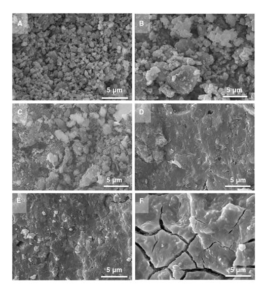
FIGURE 9. SEM images of geopolymers formulated with an  $Na_2O/SiO_2$  molar ratio of 0.25, and  $SiO_2/Al_2O_3$  molar ratios of (A) 2.0 (B) 2.2 (C) 2.4 (D) 2.6, (E) 2.8 and (F) 3.0.
