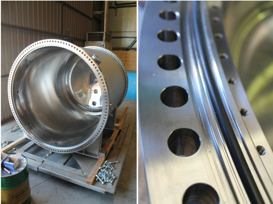
Figure 9.2.3: Exterior of NEXT-100 pressure vessel in the final stages of the construction (left). Detail of one of the gaskets used to hold the vacuum and pressure need in NEXT (right).
