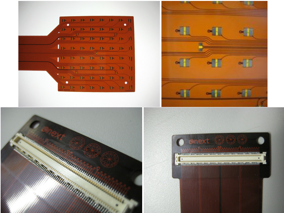
Figure 9.2.6: Picture of the DICE board to be used in the NEXT-100 detector. The material used is cirlex ® that allows for an improved soldering protocol and gives more flexibility in the design. The DICE and the first stage of the cable are now part of the same unit resulting in a better signal transmission.
