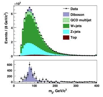
FIG. 4 (color online). Dijet invariant mass distribution with fit results overlaid for events passing all selection criteria (top) and the same background-subtracted distribution with the fitted diboson contribution overlaid (bottom). The last bin includes overflow events with  $m_{ij} > 400 \text{ GeV}/c^2$ .
