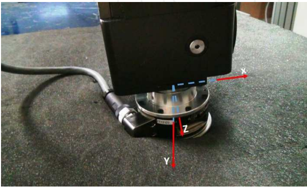
Figure 7. Reference system of the force sensor on Kraft performing a sliding effort.
