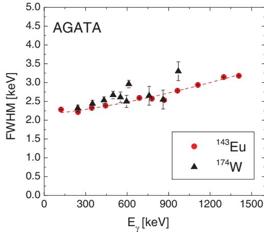
FIG. 1. (Color online) Full width at half maximum (FWHM) as a function of  $\gamma$ -ray energy, as obtained for the entire AGATA array from an  $^{143}\text{Eu}$  source (circles) and the ground-state band of  $^{174}\text{W}$ , populated in-beam in the present reaction (triangles). The dashed line is a linear fit of the  $^{143}\text{Eu}$  source data.
